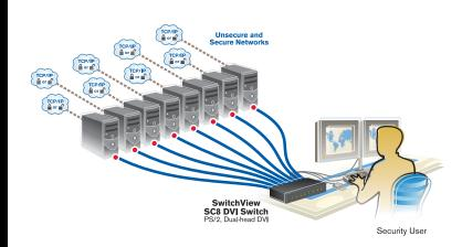
This diagram reflects how the SwitchView SC8 DVI switch supports dual-head digital and analog video applications. The DVI video lets you view multiple applications with crisp, clear resolution.
